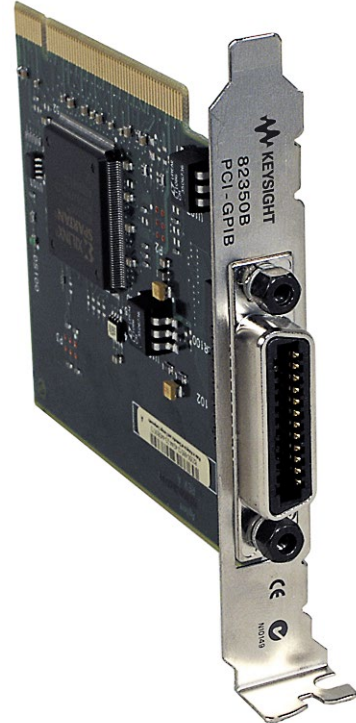
82350B PCI high-performance GPIB interface card
